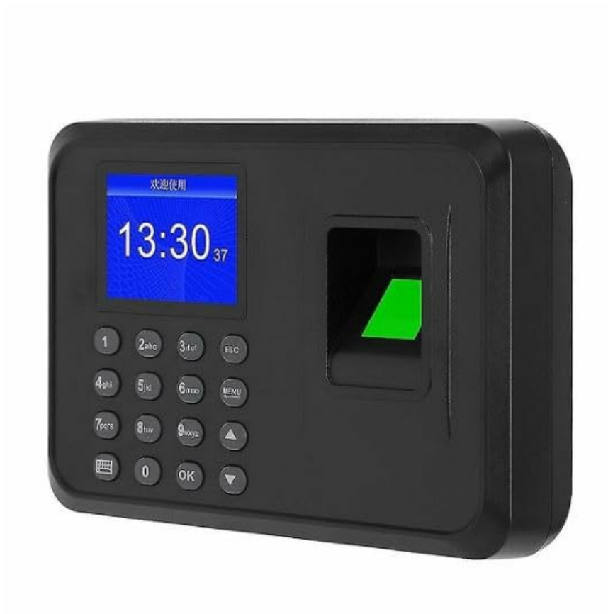
Figure 1: MY-7078 Device Front View. This image displays the device's screen, numeric keypad, and the illuminated fingerprint scanner on the right side.
