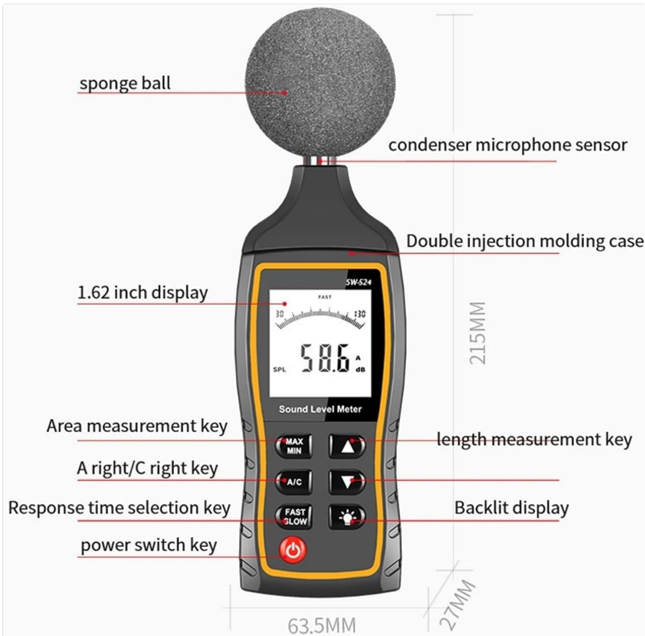
Figure 2: Labeled components and dimensions of the SW-524.
