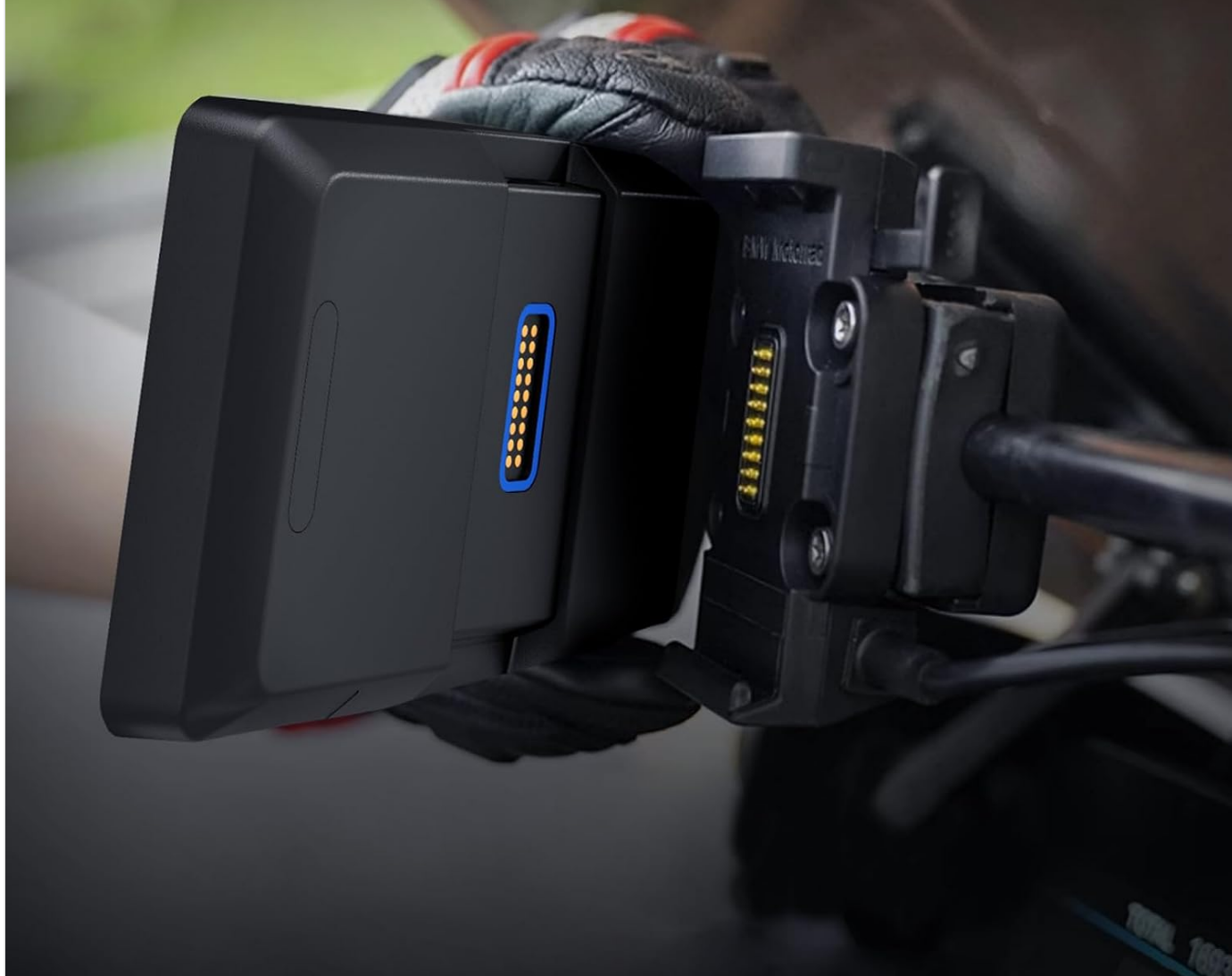
Figure 1: CARABC DB601 device with 3-pin connector for BMW integration.
