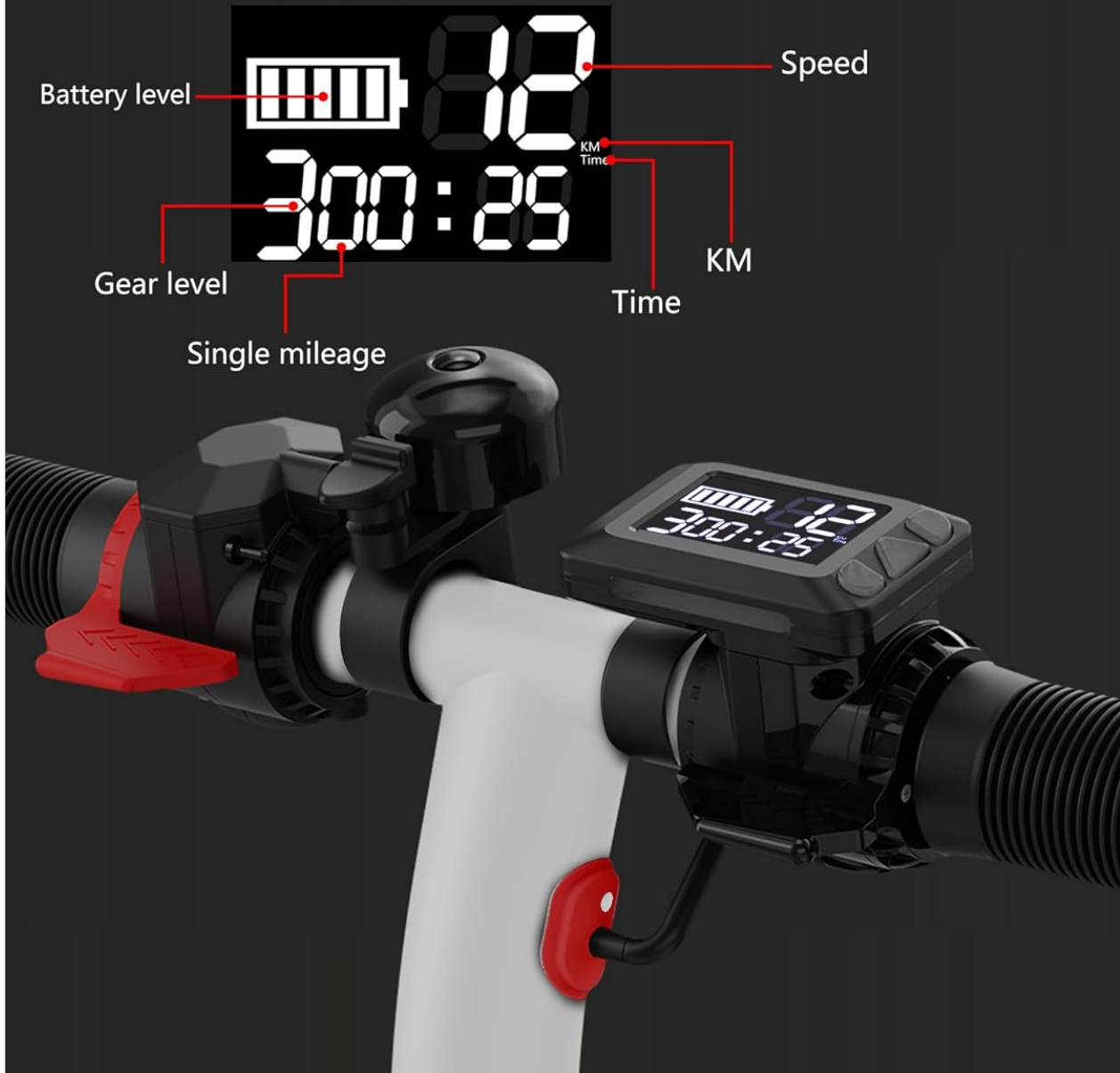
Image 5.1: LED Display. A detailed view of the handlebar-mounted LED display, indicating current battery charge, speed, selected gear mode, and trip distance.
