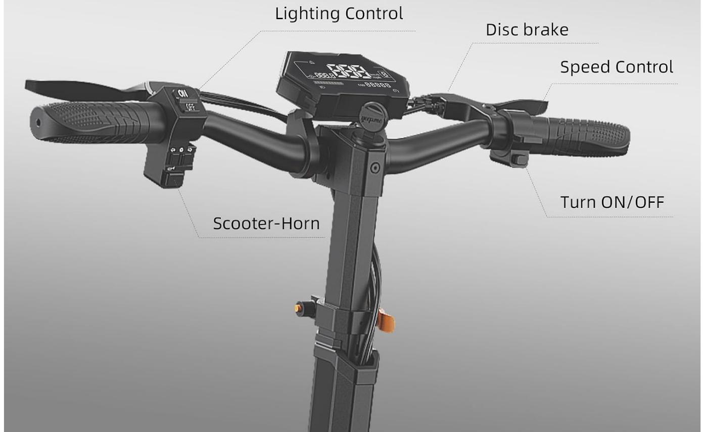
Figure 5.1: The Smart LED Display and handlebar controls, including lighting control, disc brake, speed control, and horn.
