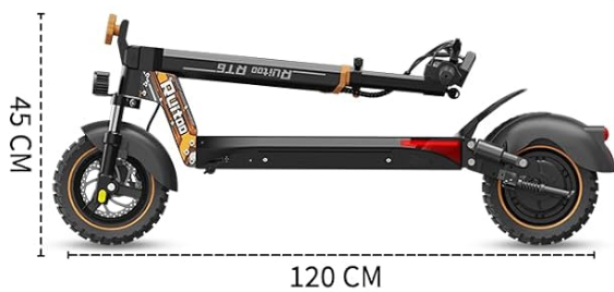
Figure 4.1: The RT6 scooter in its folded state, demonstrating its portability for storage or transport.
