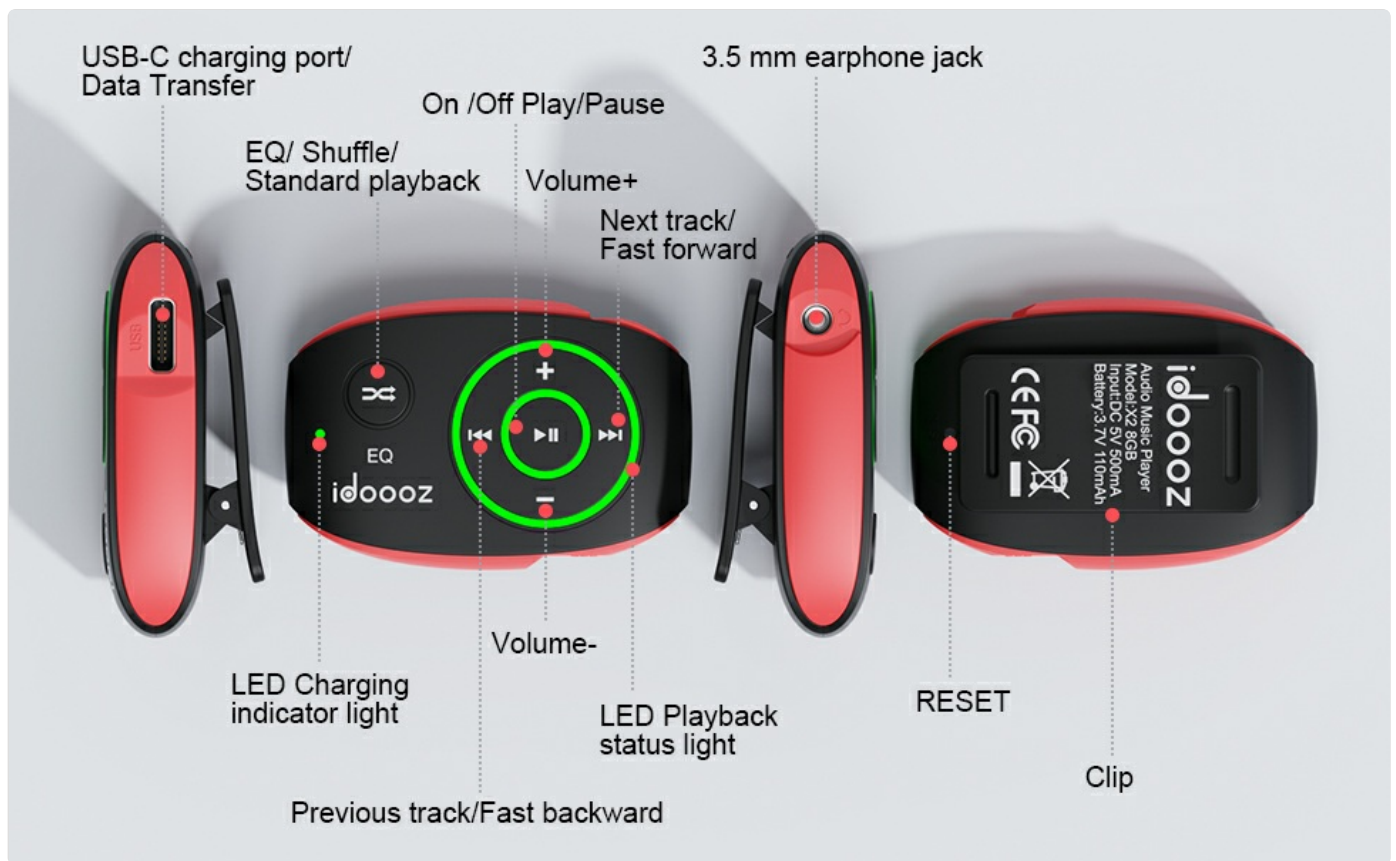
Image 3.1: Labeled diagram of the idooz X2 MP3 Player components.
