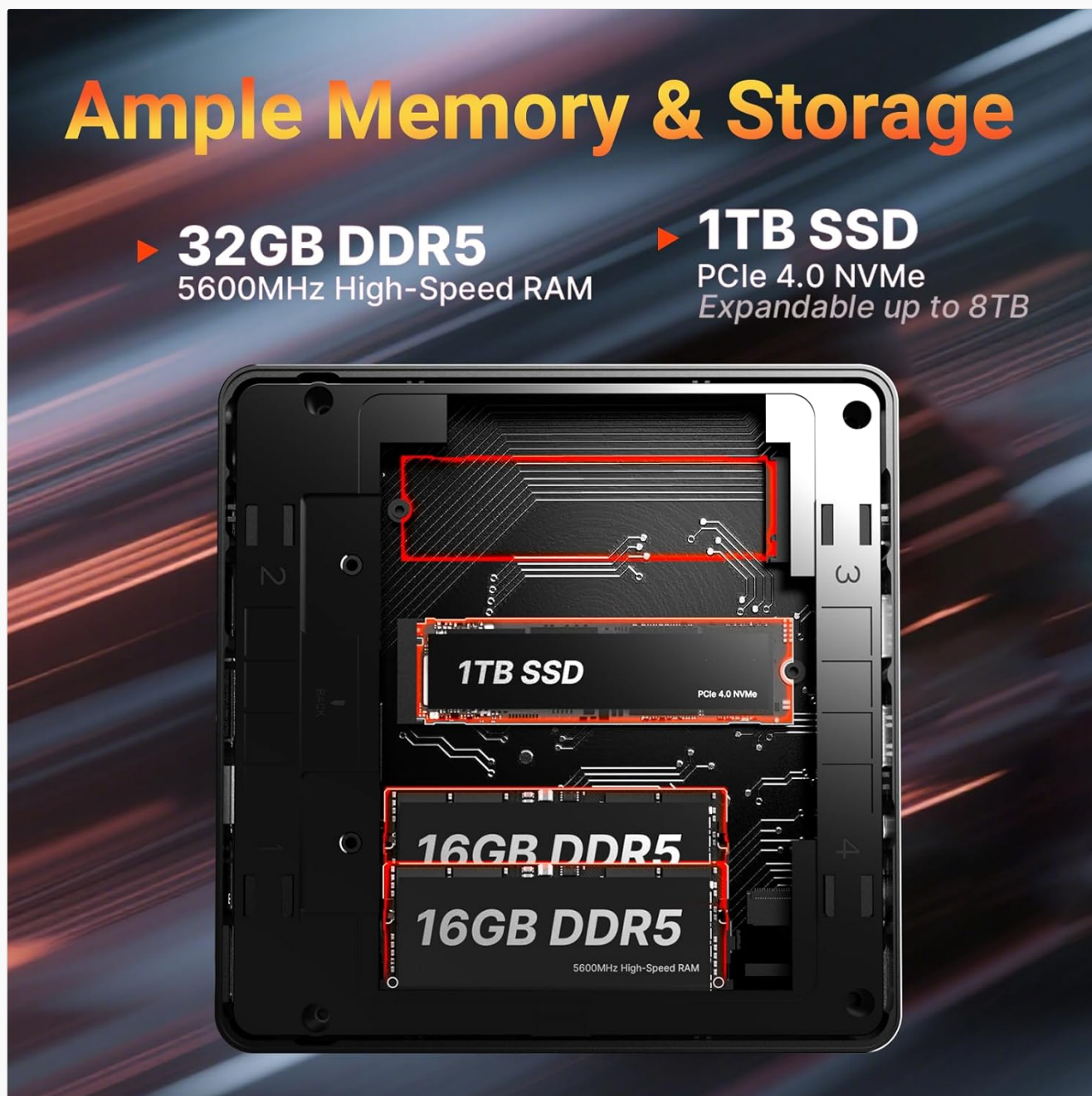
Image 5.2: Ample Memory & Storage. The Mini PC supports 32GB DDR5 RAM and a 1TB PCIe 4.0 NVMe SSD, with expansion options.
