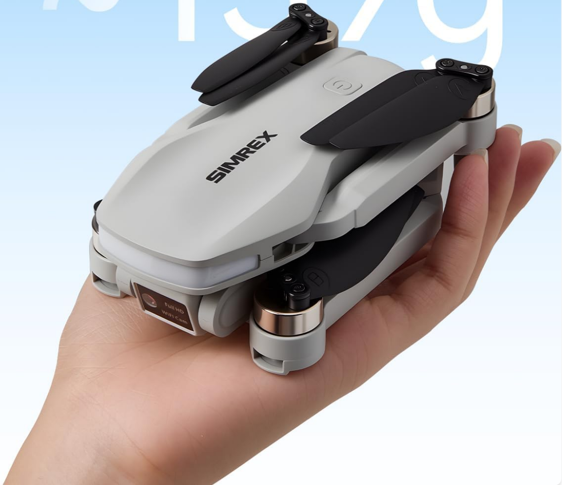
Image 6.2: The drone's foldable design and lightweight nature (approximately 139g).
