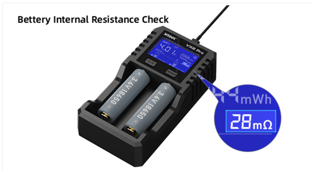
Image 4.7.1: The charger's display indicating the internal resistance (IR) measurement for a battery.
