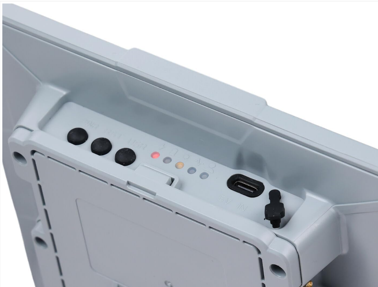
Figure 3: Side view of the SenseCAP Solar Node P1-Pro showing USB-C port, power button, reset button, and LED indicators.
