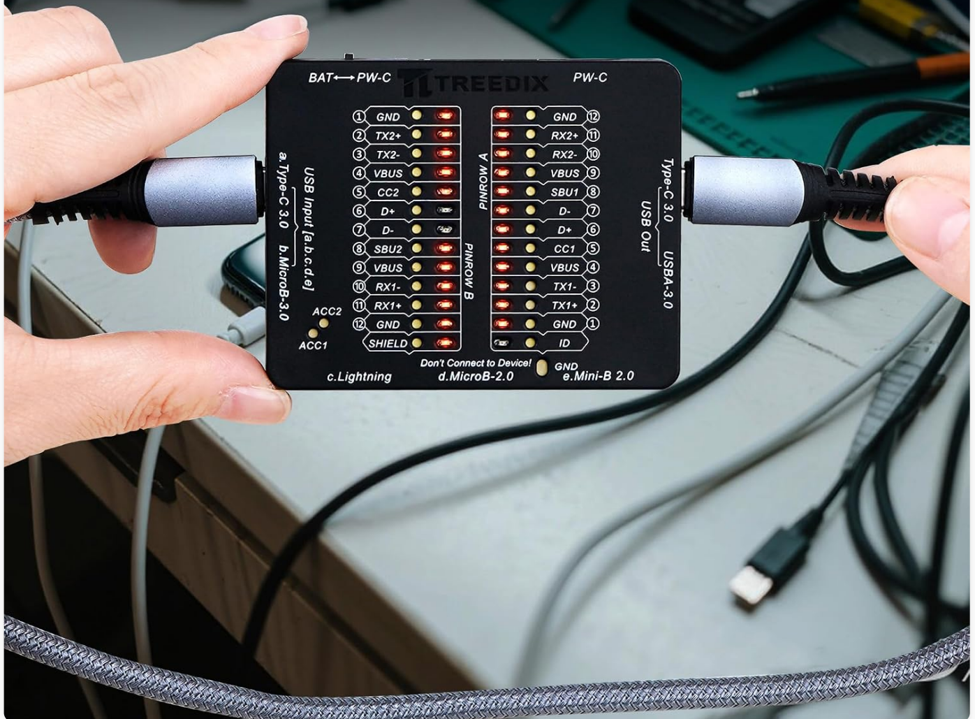
Image: A user demonstrating the Treedix USB Cable Tester in action, with a USB-C cable plugged in and the LED indicators showing connection status.
