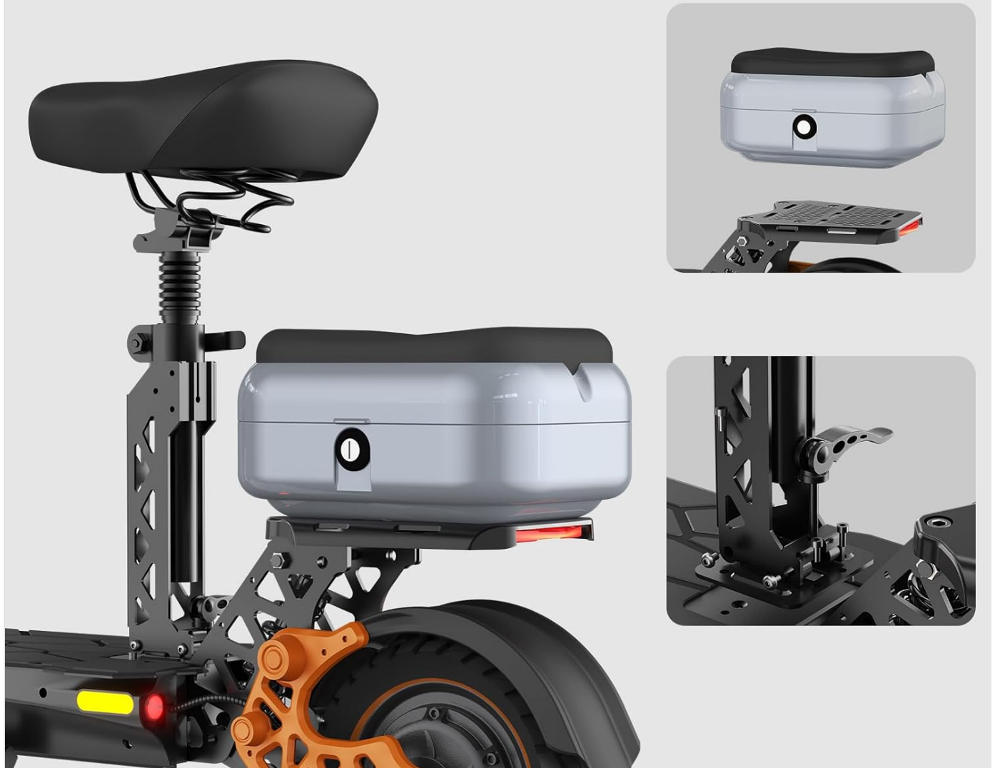
Image: Detailed view of the removable seat and storage box, illustrating how they attach to the scooter's frame.
