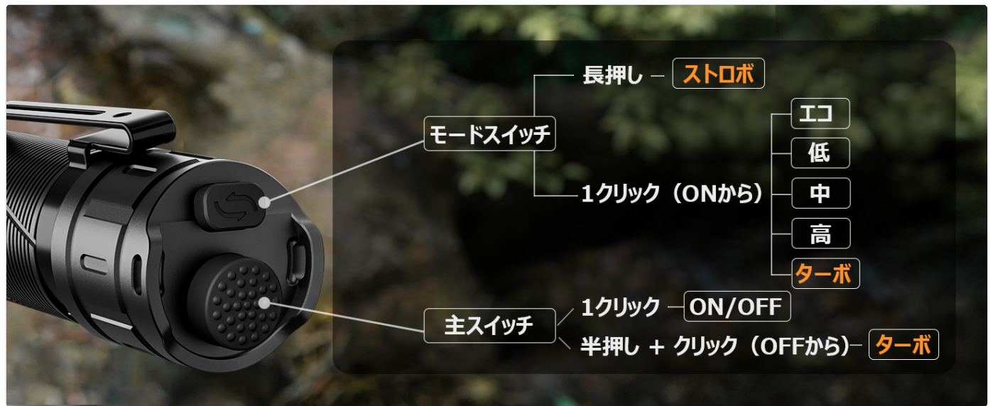
Image: Diagram illustrating the Main Switch and Mode Switch locations and their primary functions.
