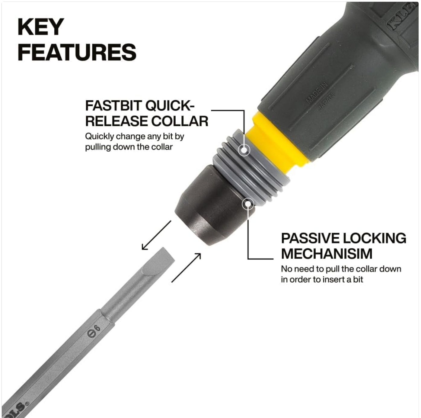
Figure 1: Fastbit Quick-Release Collar and Passive Locking Mechanism. Pull down the collar to release the bit.
