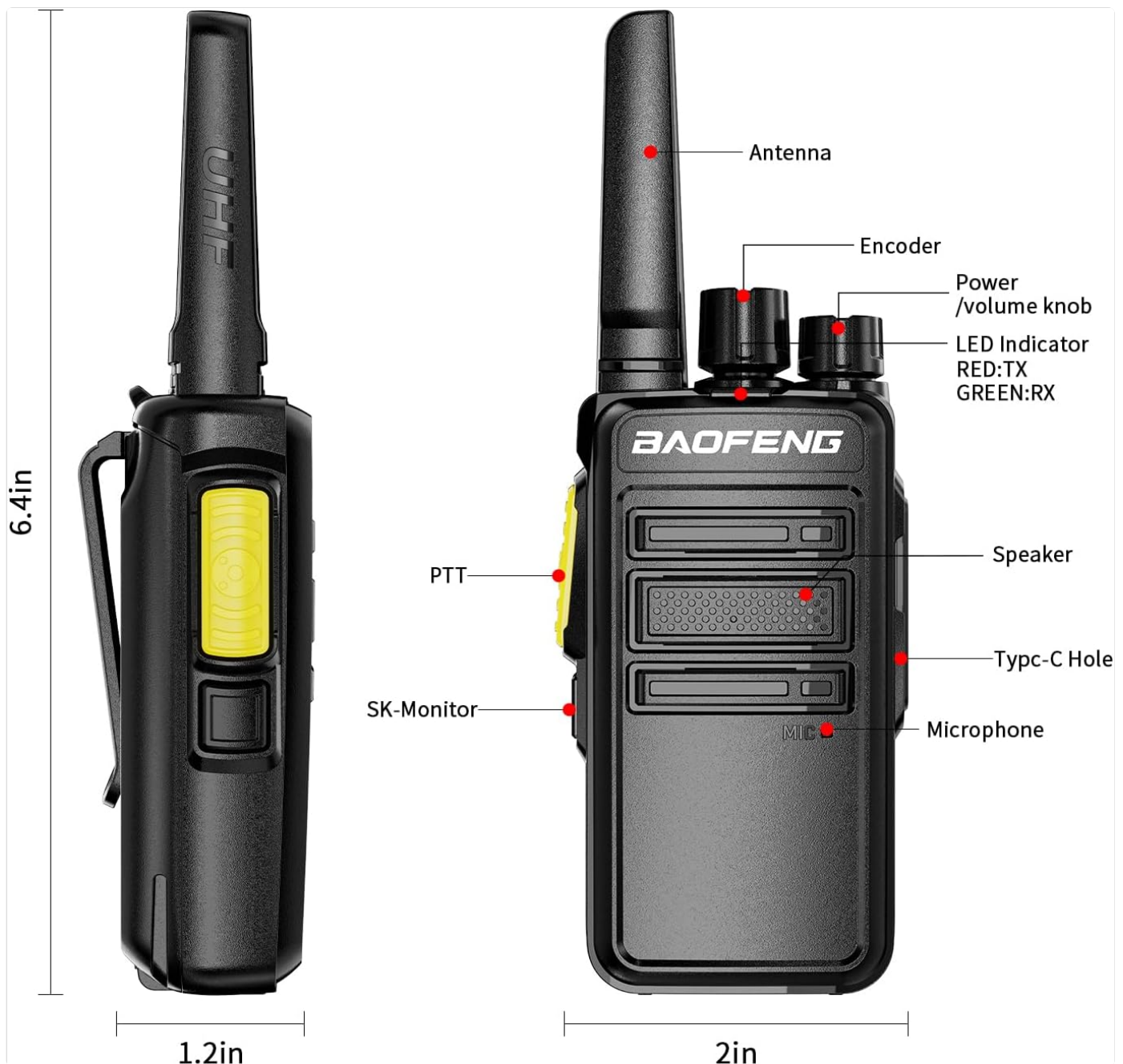
Figure 3.1: Labeled diagram of the BAOFENG BD-V12B radio. Key components include the Antenna, Encoder (channel selector), Power/Volume knob, LED Indicator (Red for TX, Green for RX), PTT (Push-to-Talk) button, SK-Monitor button, Speaker, Type-C Charging Port, and Microphone.
