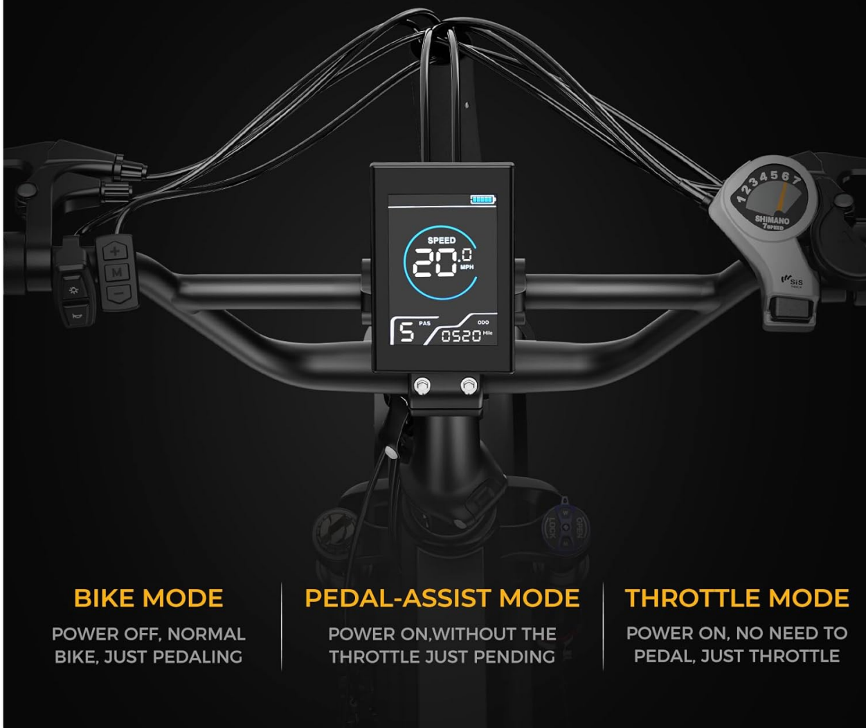
Image 4.1: The intuitive LCD display showing speed, battery charge, and pedal assist level, with controls for riding modes.
