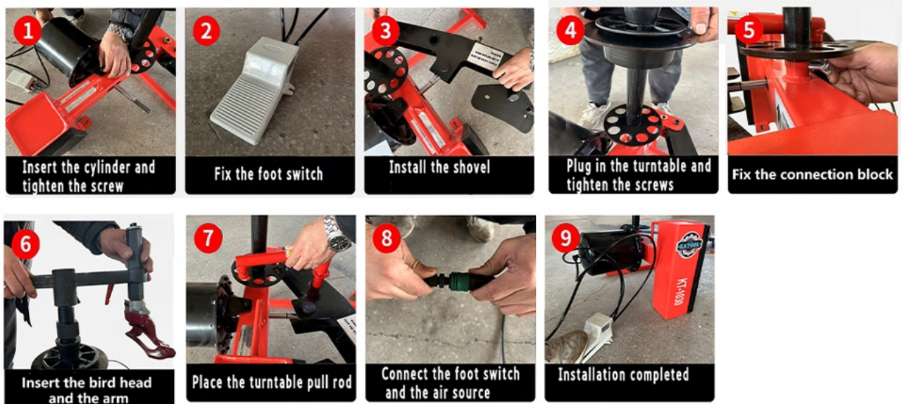
Figure 4.1: Assembly steps for the KATOOL Mini Tire Changer Machine KT-1030P.
