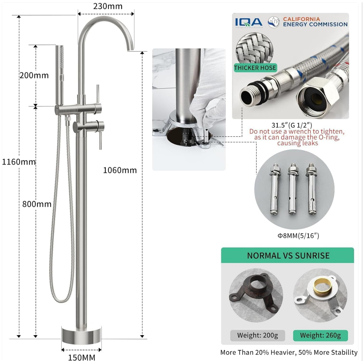
Figure 3: Faucet dimensions and important note on connection tightening.
