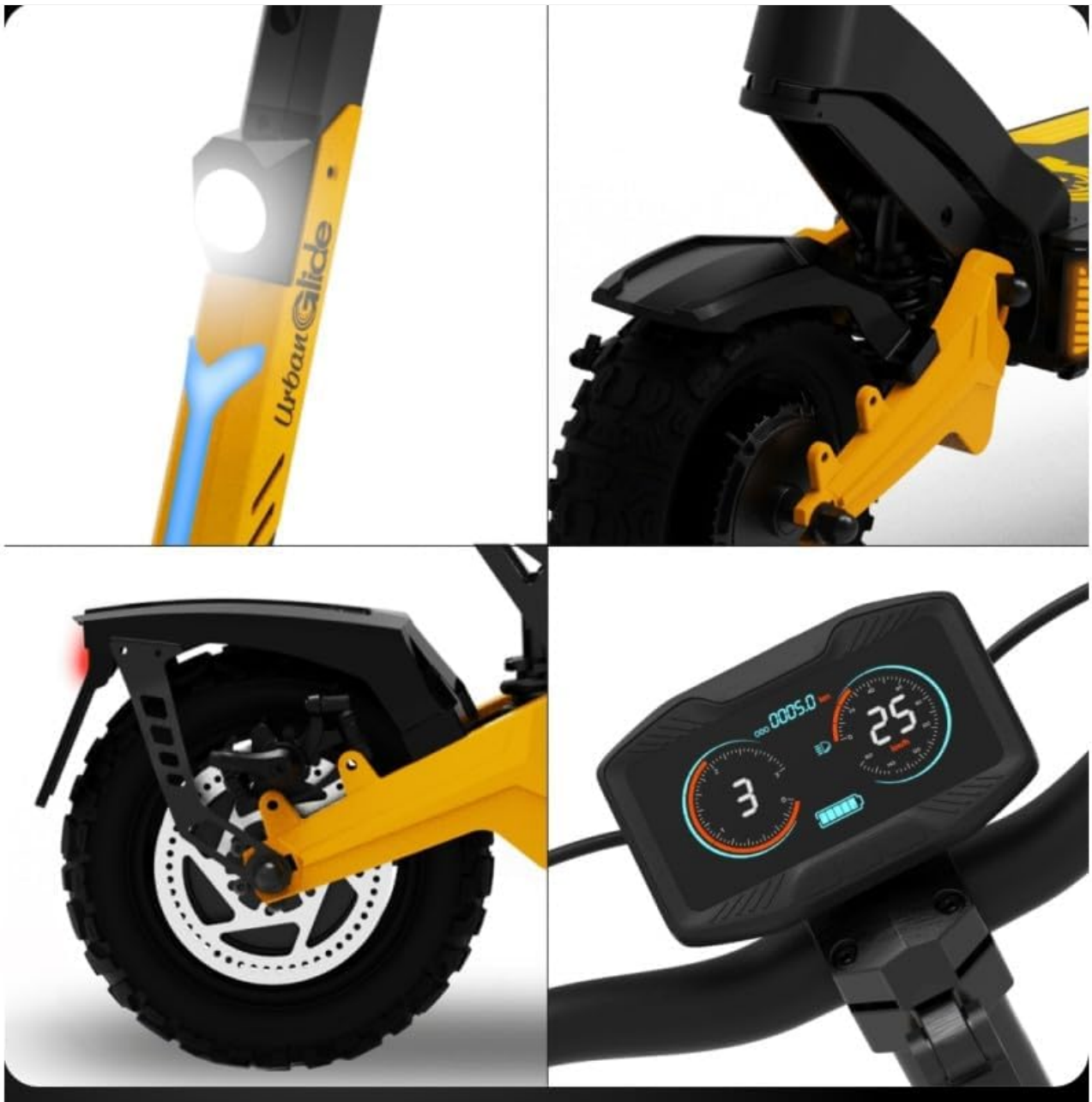
Figure 3.3: Detailed view of key components including the front headlight, rear wheel with disc brake, and the digital display showing speed and battery level.
