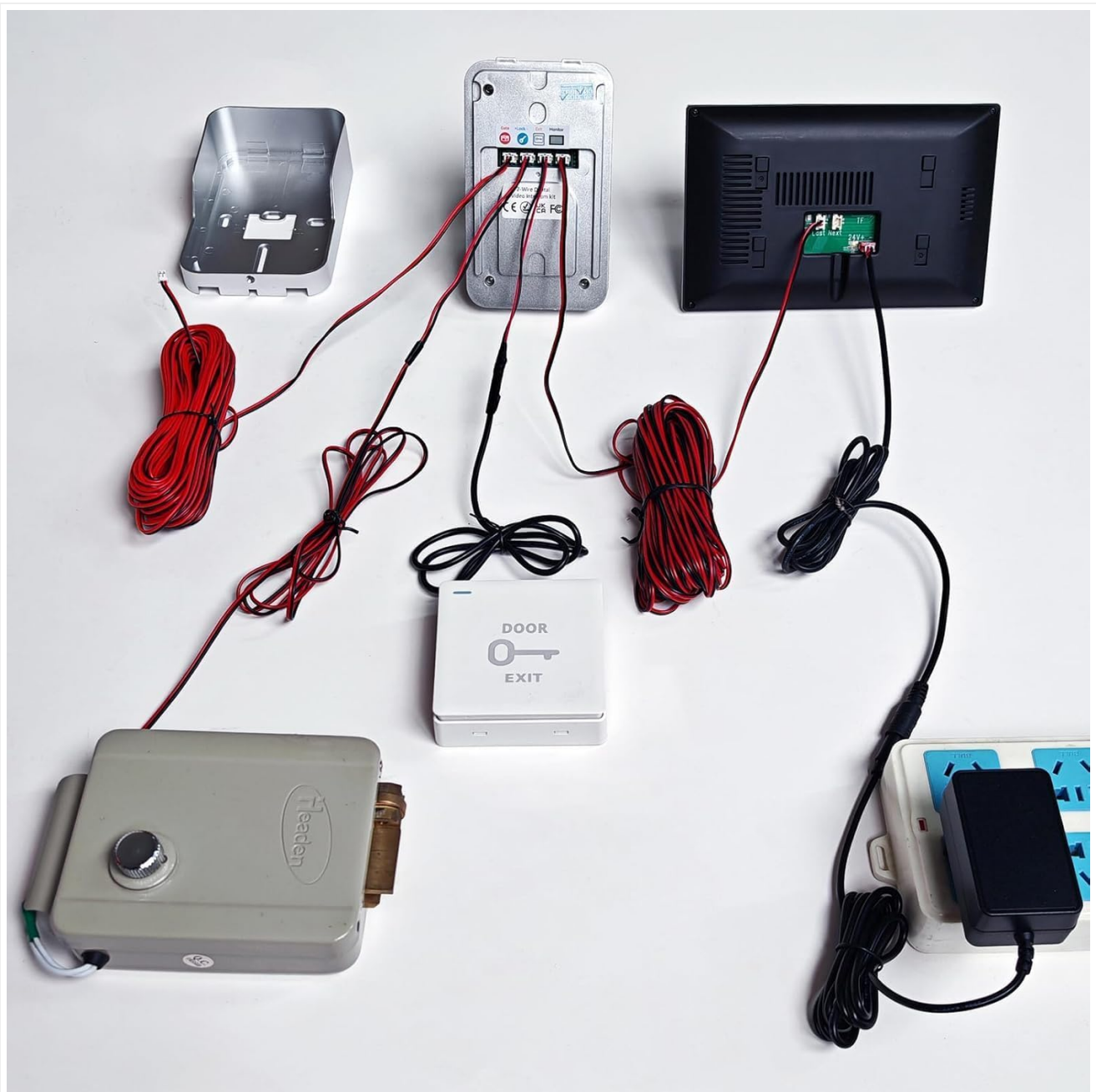
Figure 4.1: Detailed wiring diagram showing connections for the outdoor doorbell, indoor monitor, power supply, and optional door/gate controls. Note the recommended wire rod distances based on core diameter.
