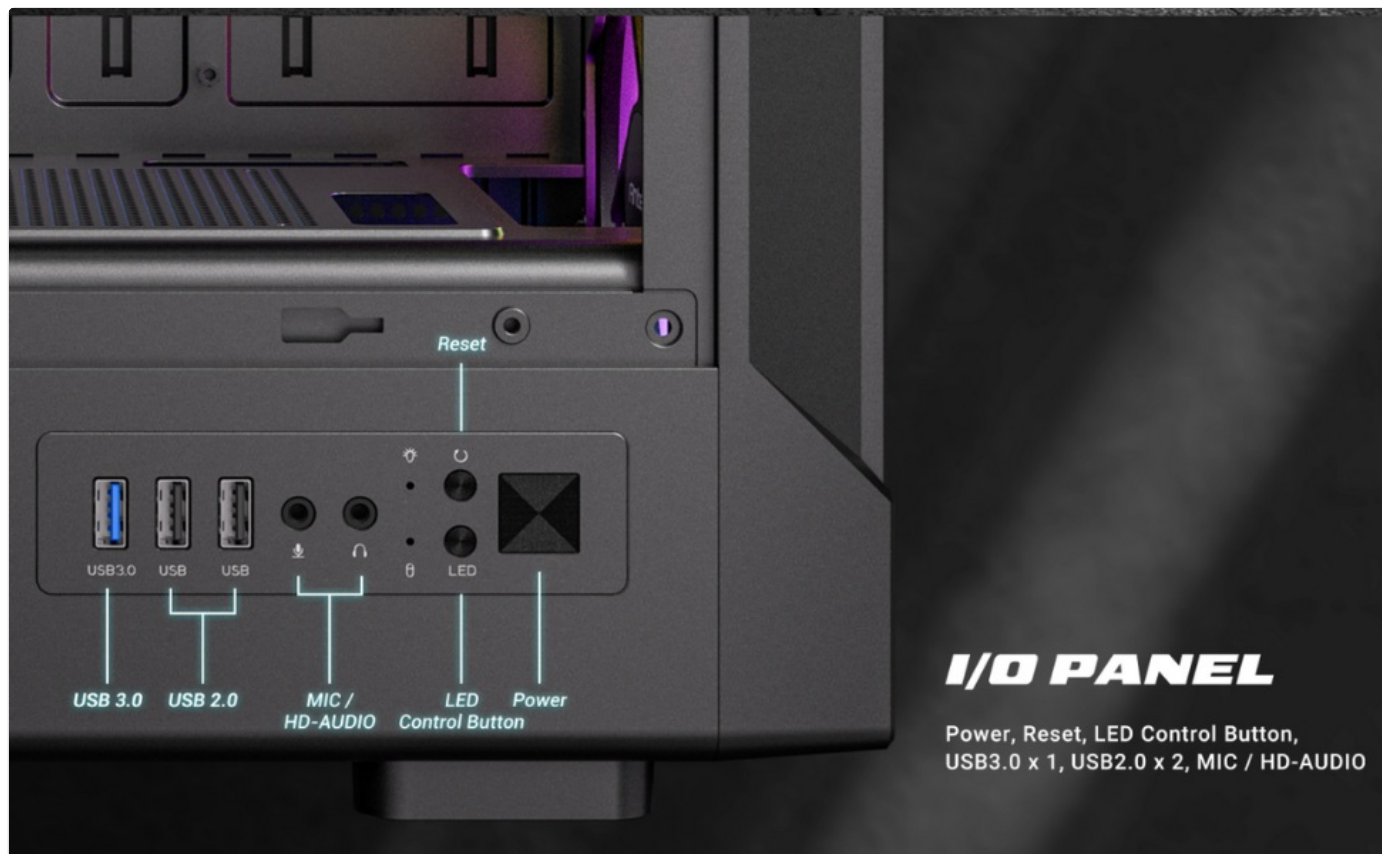
Image 4.1: The front I/O panel, showing the location of USB 3.0, USB 2.0, audio jacks, LED control, reset, and power buttons. Ensure these are correctly connected to your motherboard.
