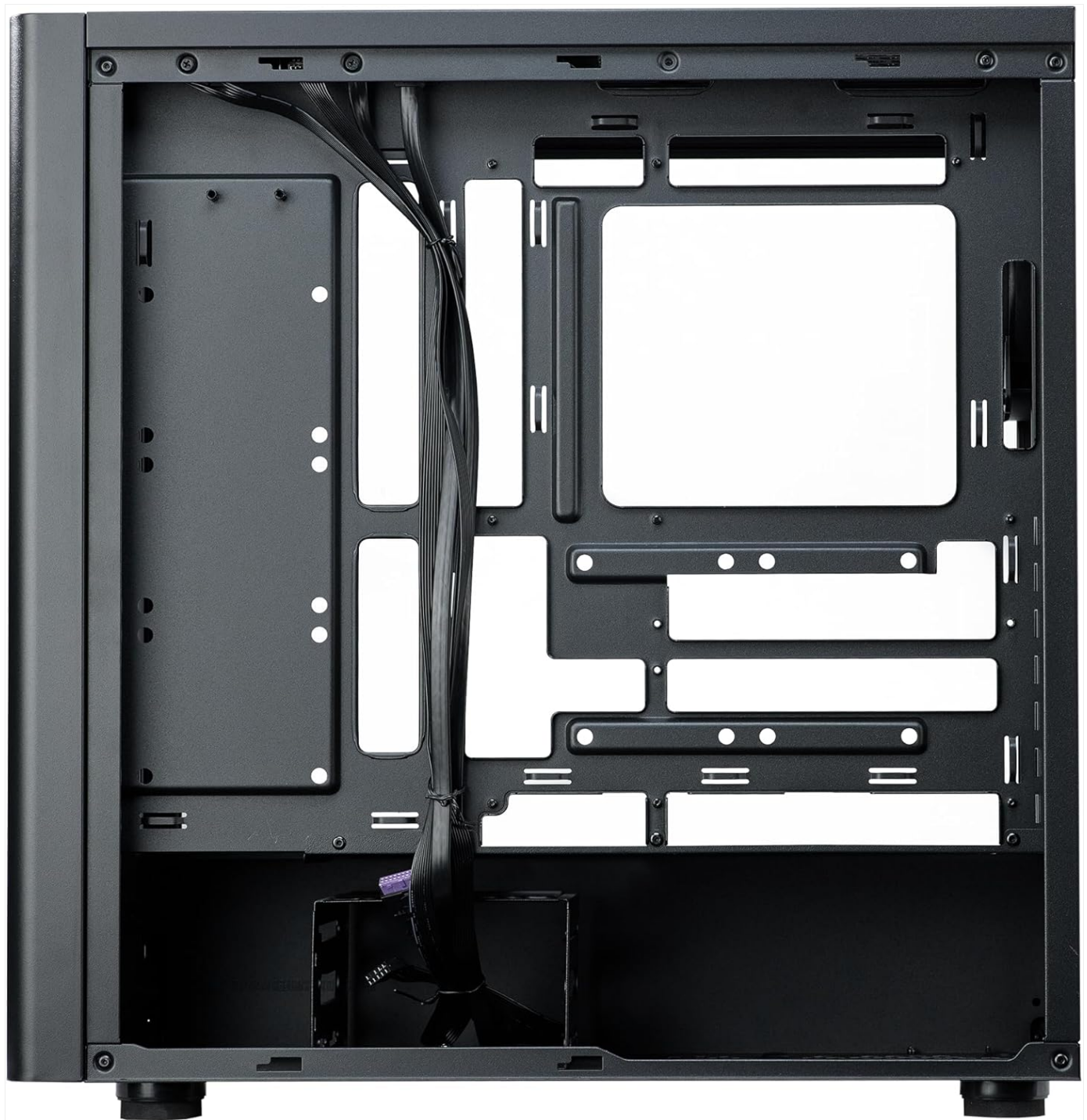
Figure 4.7: Rear interior view of the case, showing the space and tie-down points available for effective cable management behind the motherboard tray. This helps maintain a clean build and optimize airflow.
