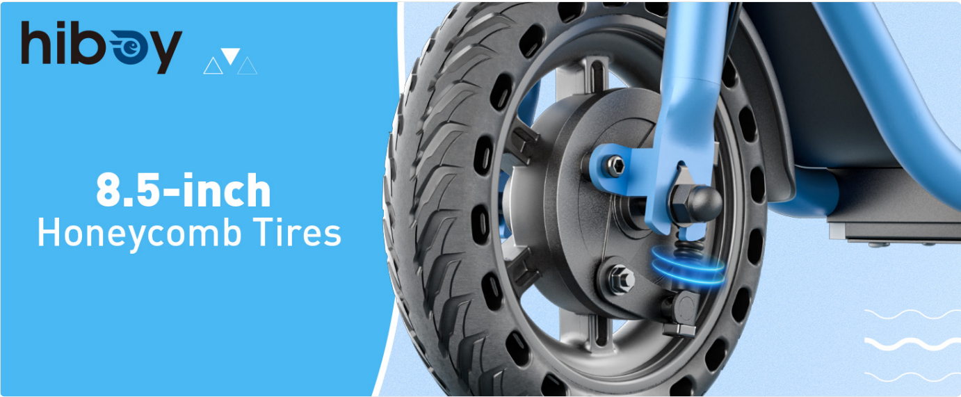
Image: Close-up view of the scooter's 8.5-inch honeycomb tires, highlighting their solid construction.
