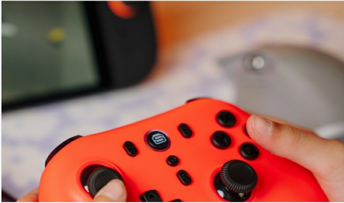
Figure 2: The controller highlighting its Hall Effect Thumb Sticks and Triggers for enhanced precision.
