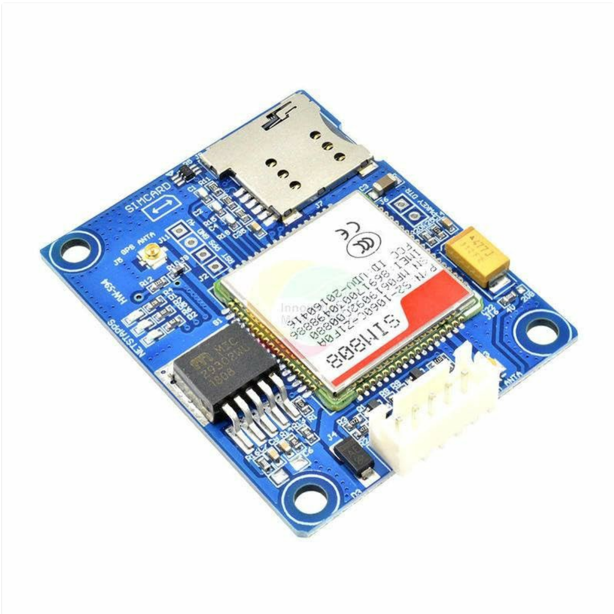
Figure 4: Angled view of the module, indicating the locations for antenna connections.
