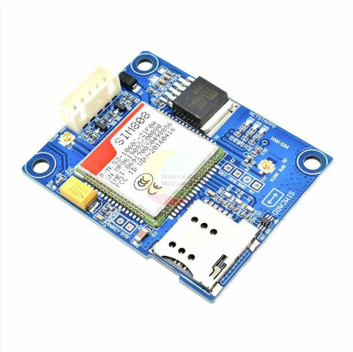
Figure 3: Angled view of the module, clearly showing the TF card slot and SIM card slot.
