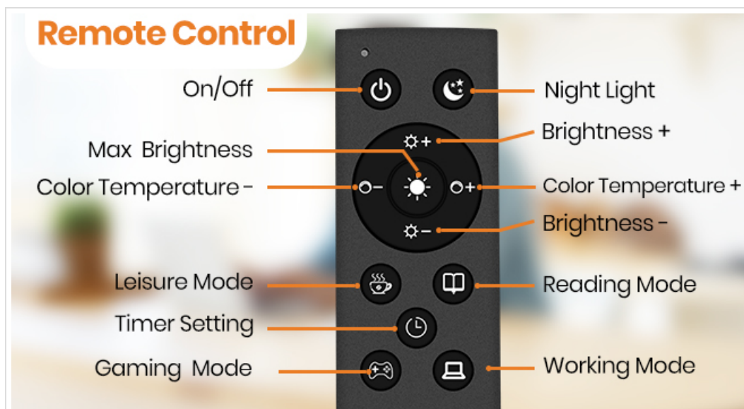
Image: Detailed layout of the remote control with button descriptions.
