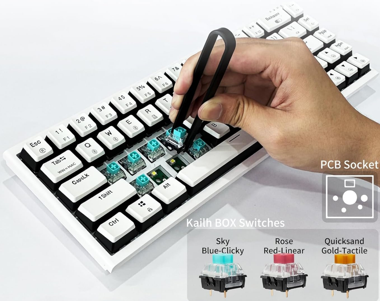
Image 3.3: A switch being removed from the Hexgears X1 Pro keyboard using a switch puller, demonstrating the hot-swappable feature.
