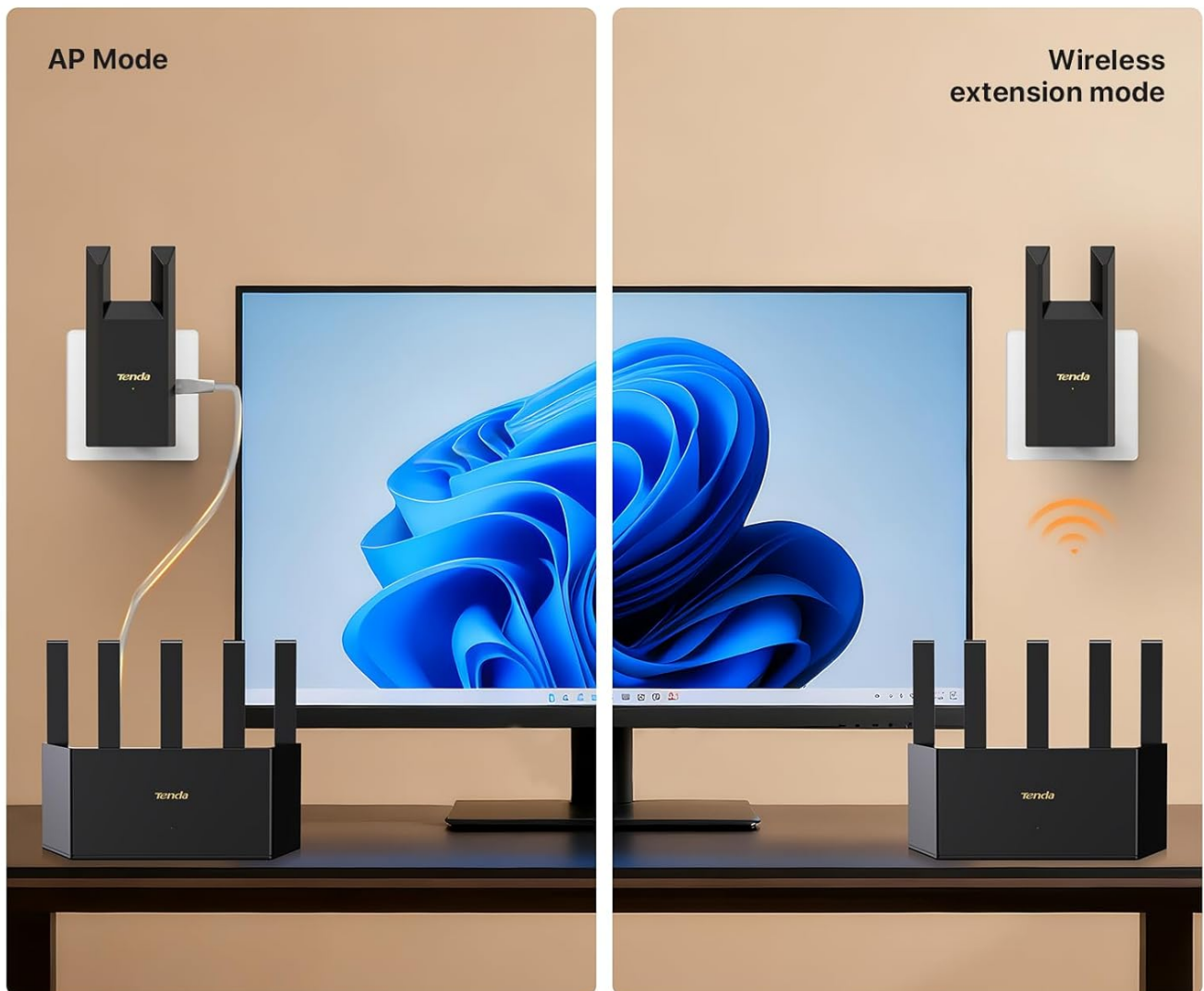
Figure 3: AP Mode and Wireless Extension Mode
