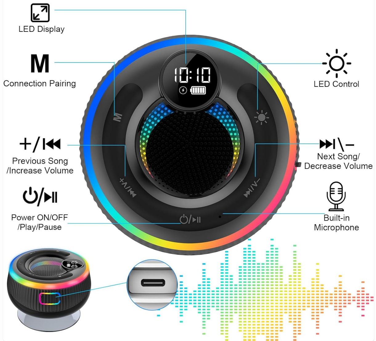
Image 3: Detailed view of the speaker's buttons and their corresponding functions.
