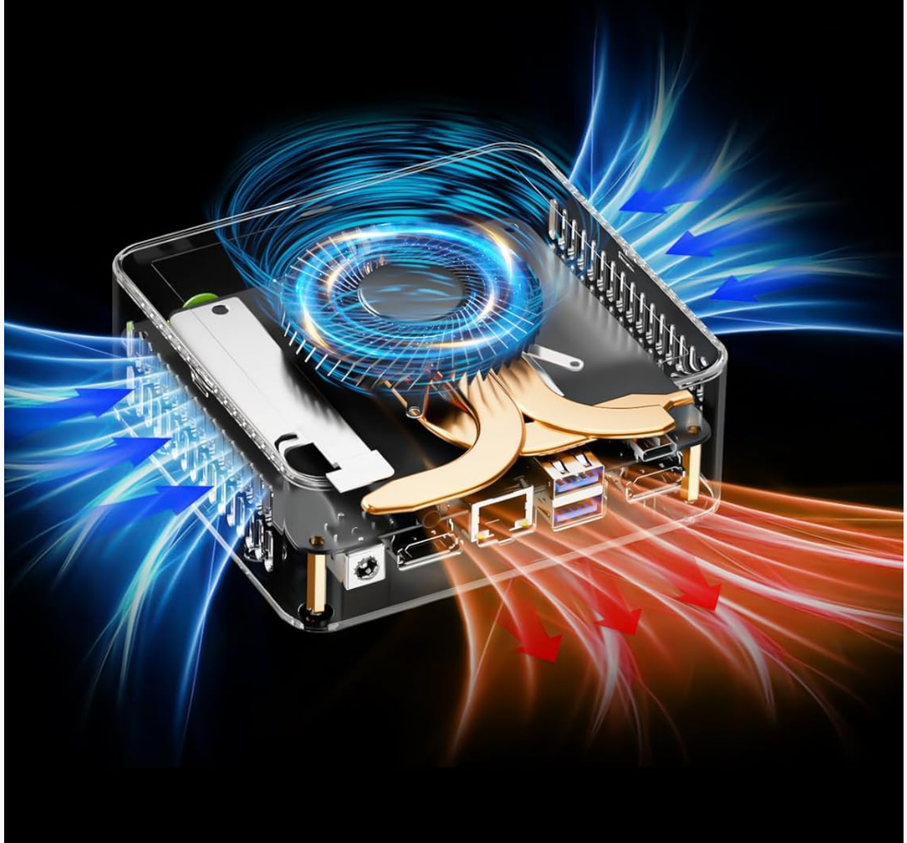
Image: Diagram illustrating the dual turbo cooling, two-way convection air inlet, and quiet cooling design of the GMKtec Mini PC M3 Ultra.
