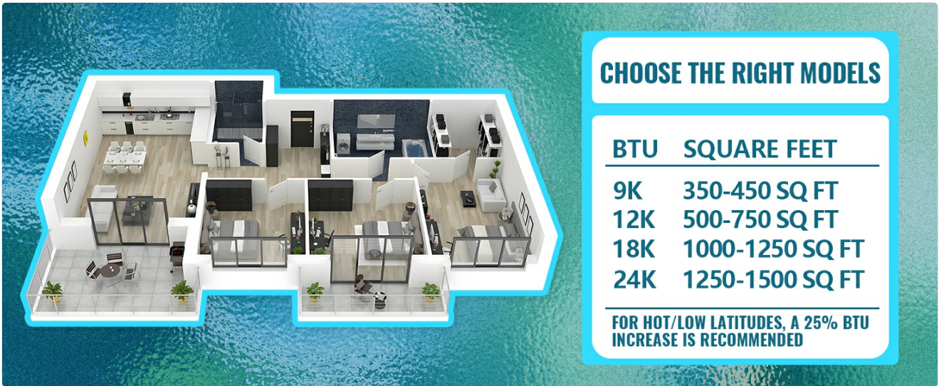
Image: A guide illustrating recommended BTU capacities for different square footage areas, from 9K BTU for 350-450 sq ft to 24K BTU for 1250-1500 sq ft.
