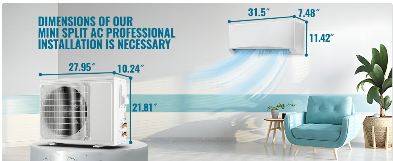
Image: Diagram showing the dimensions of the indoor unit (31.5"W x 7.48"D x 11.42"H) and the outdoor unit (27.95"W x 10.24"D x 21.81"H), crucial for planning installation space.
