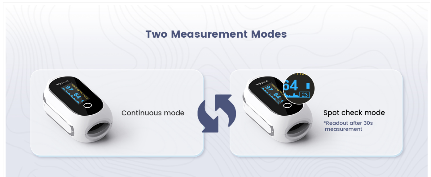
Image 5.2: Illustration of the two measurement modes: Continuous and Spot Check.
