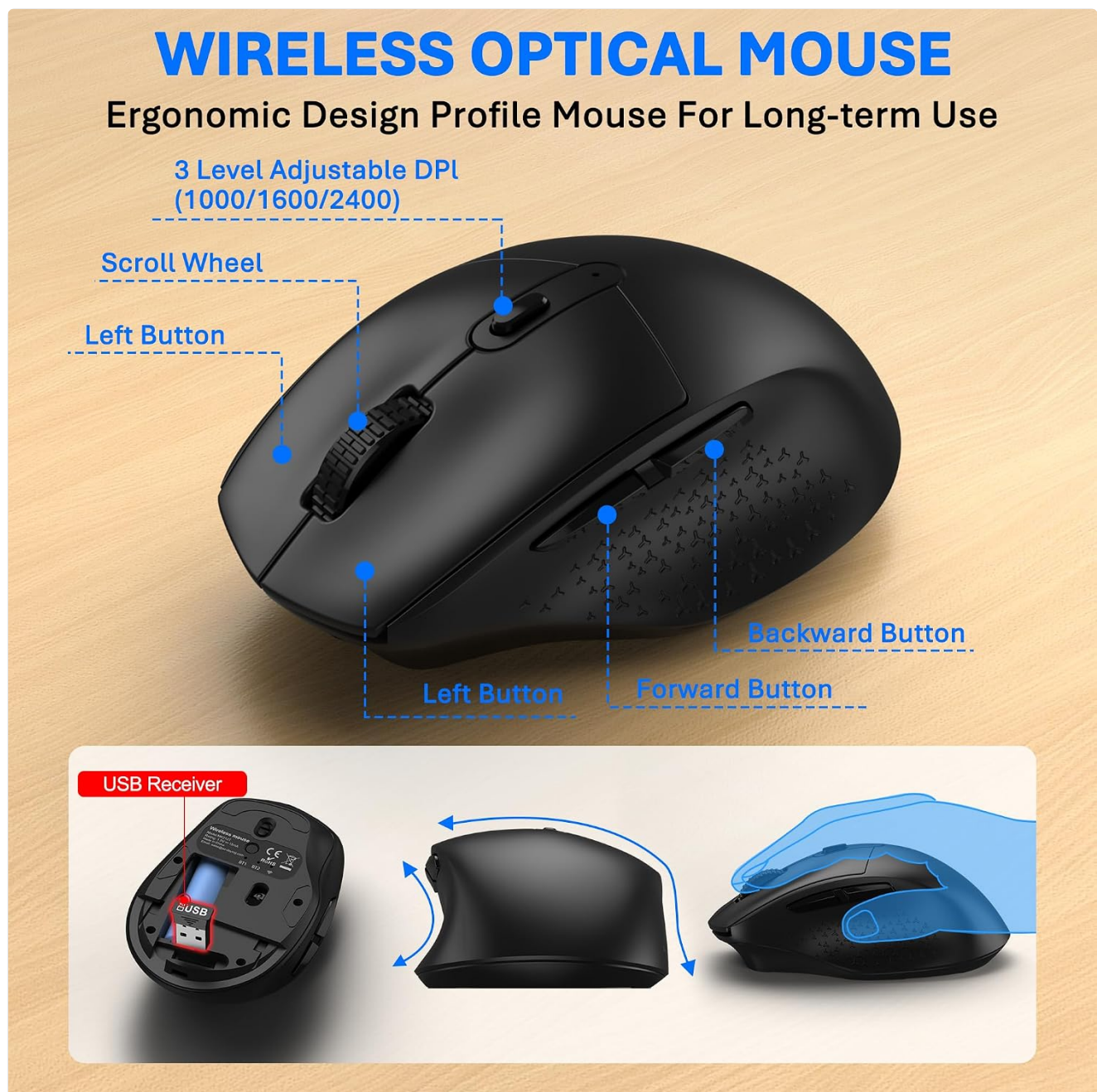
Image 3.1: Detailed view of the wireless mouse, highlighting the USB receiver storage compartment.
