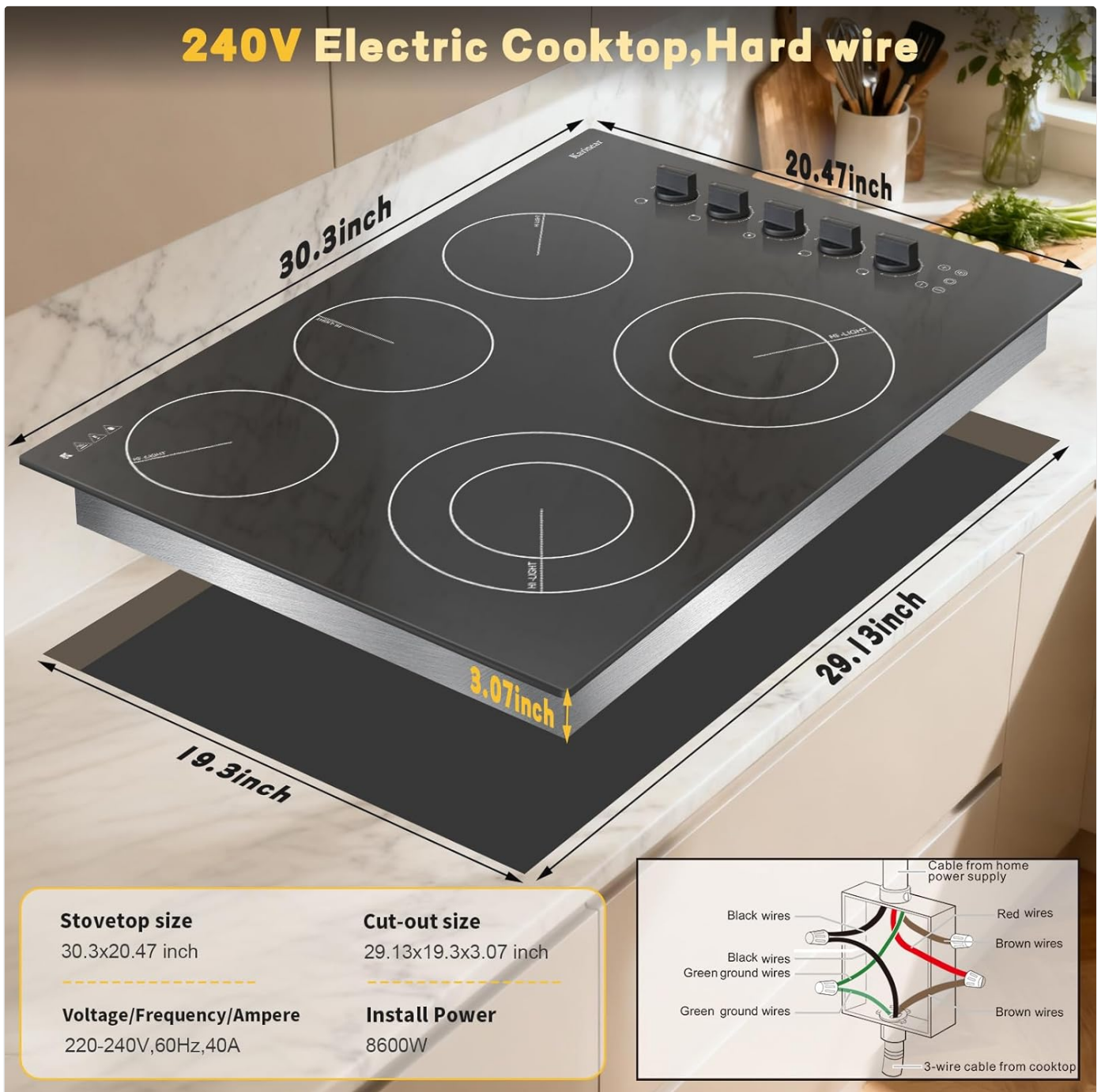
Figure 4.1: Cooktop dimensions and a diagram illustrating the 240V hardwiring connection.
