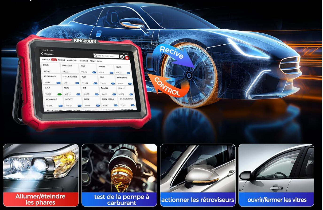
Figure 4.2: Illustration of the bi-directional control feature, showing the ability to activate various vehicle components like ABS motor pump, cooling fan, and window/mirror operations directly from the tablet.
