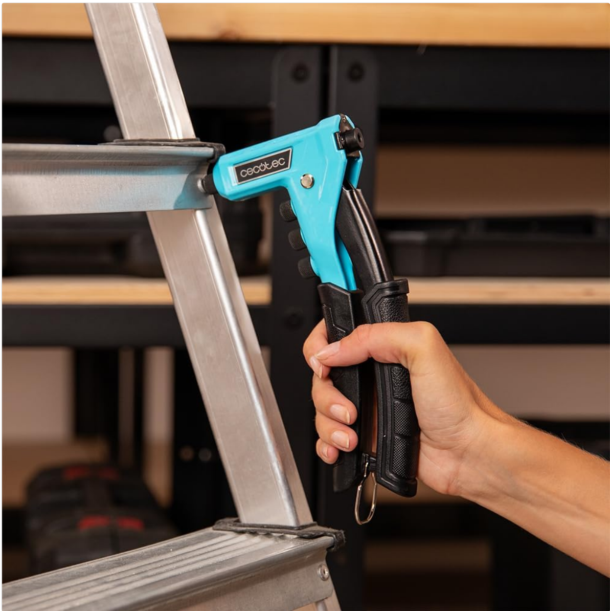
Image 5.1: Demonstrating the use of the riveter on a metal structure.
