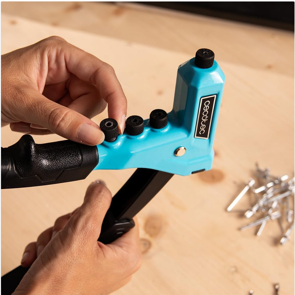
Image 4.1: Adjusting the nozzle on the riveter head.
