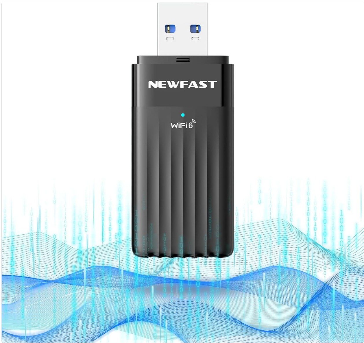
Image 1.1: The NEWFAST NF-U351 AX3000 USB 3.0 WiFi 6 Adapter, a compact black device with a USB 3.0 connector.
