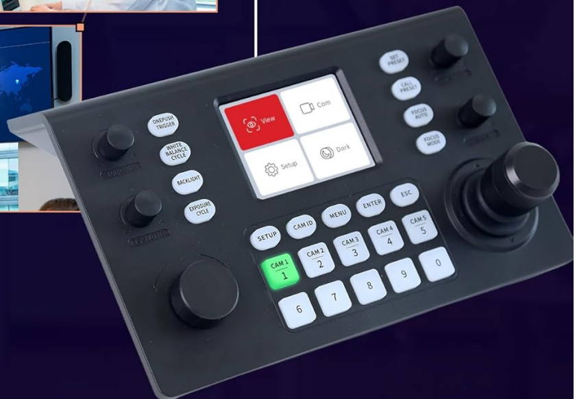
Image 2.4: NDI|HX camera search and control interface on the controller.
