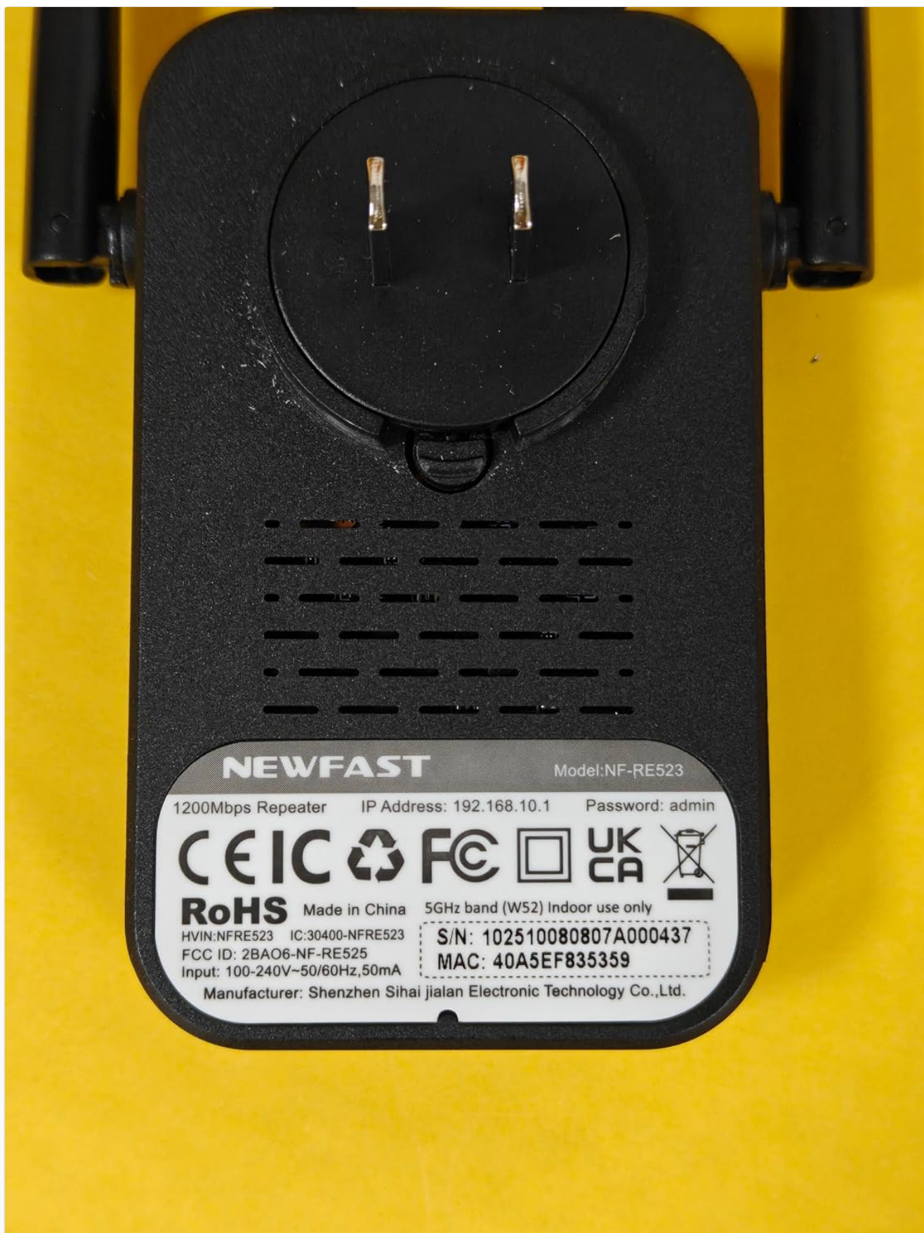
Image 3.2: Back view of the NEWFAST NF-RE523 WiFi Repeater, showing the power plug, ventilation, and product label with model and network details.
