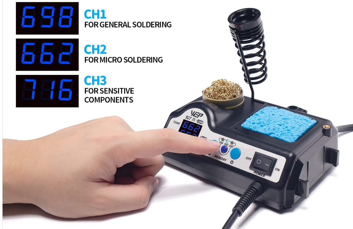
Figure 6.2: Customizing and recalling temperature settings with 3 channels.
