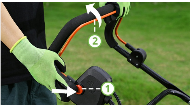
Image: Close-up of the handle showing the two-step starting process: press safety button (1), then pull operating lever (2).
