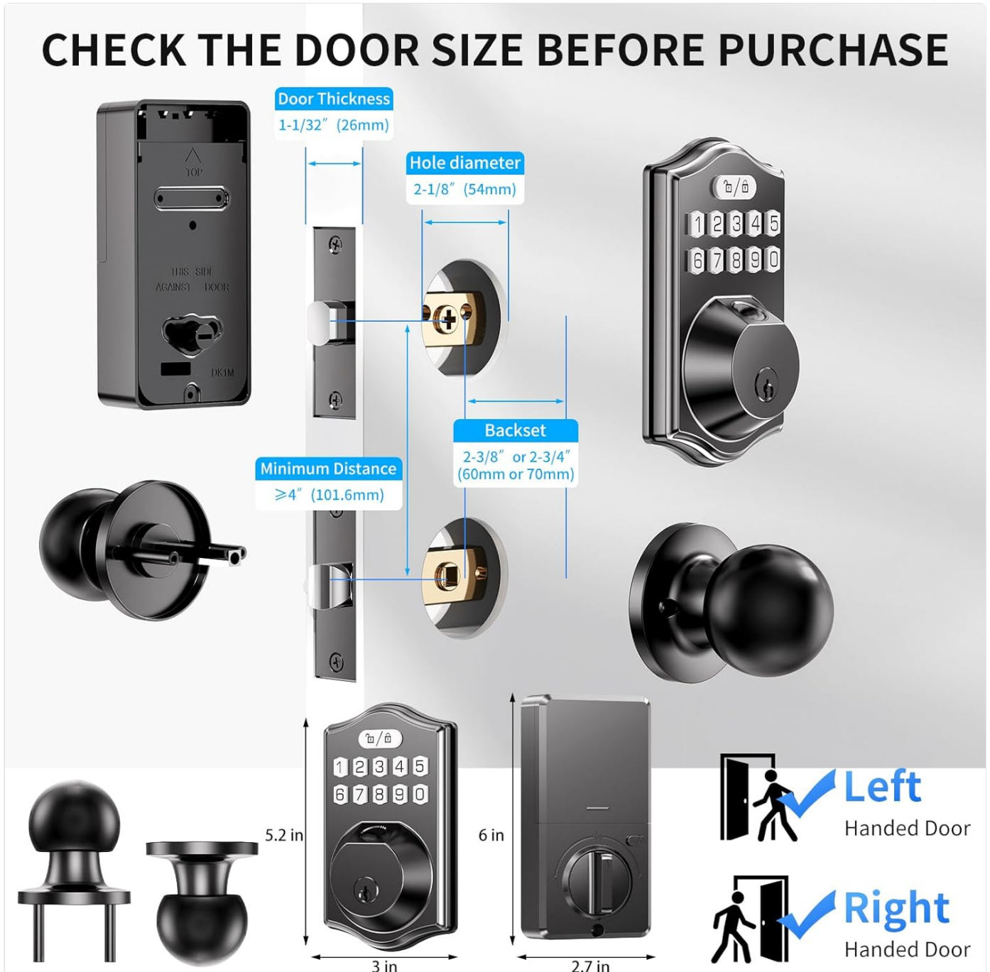
Figure 5.1: Door Size Check. This diagram illustrates critical door measurements for compatibility: Door Thickness (1-1/32" to 26mm), Hole Diameter (2-1/8" or 54mm), Backset (2-3/8" or 2-3/4", 60mm or 70mm), and Minimum Distance (≥4" or 101.6mm). It also shows the lock dimensions and suitability for both left and right-handed doors.
