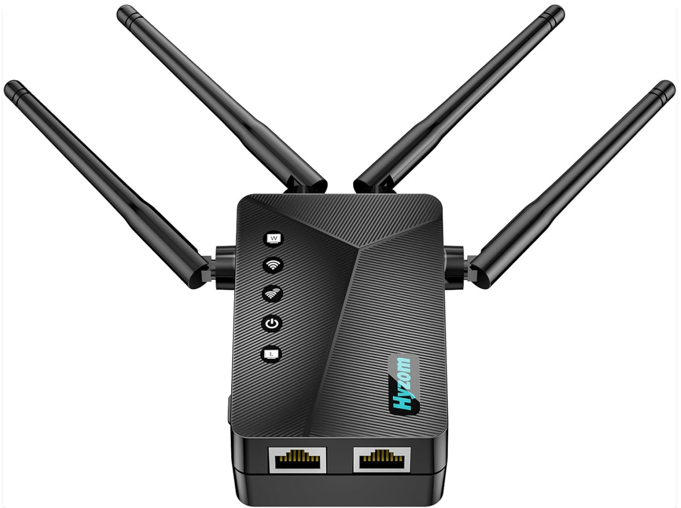
Figure 1: The Hyzom WiFi Extender Booster, showcasing its four adjustable antennas and dual Ethernet ports at the bottom.
