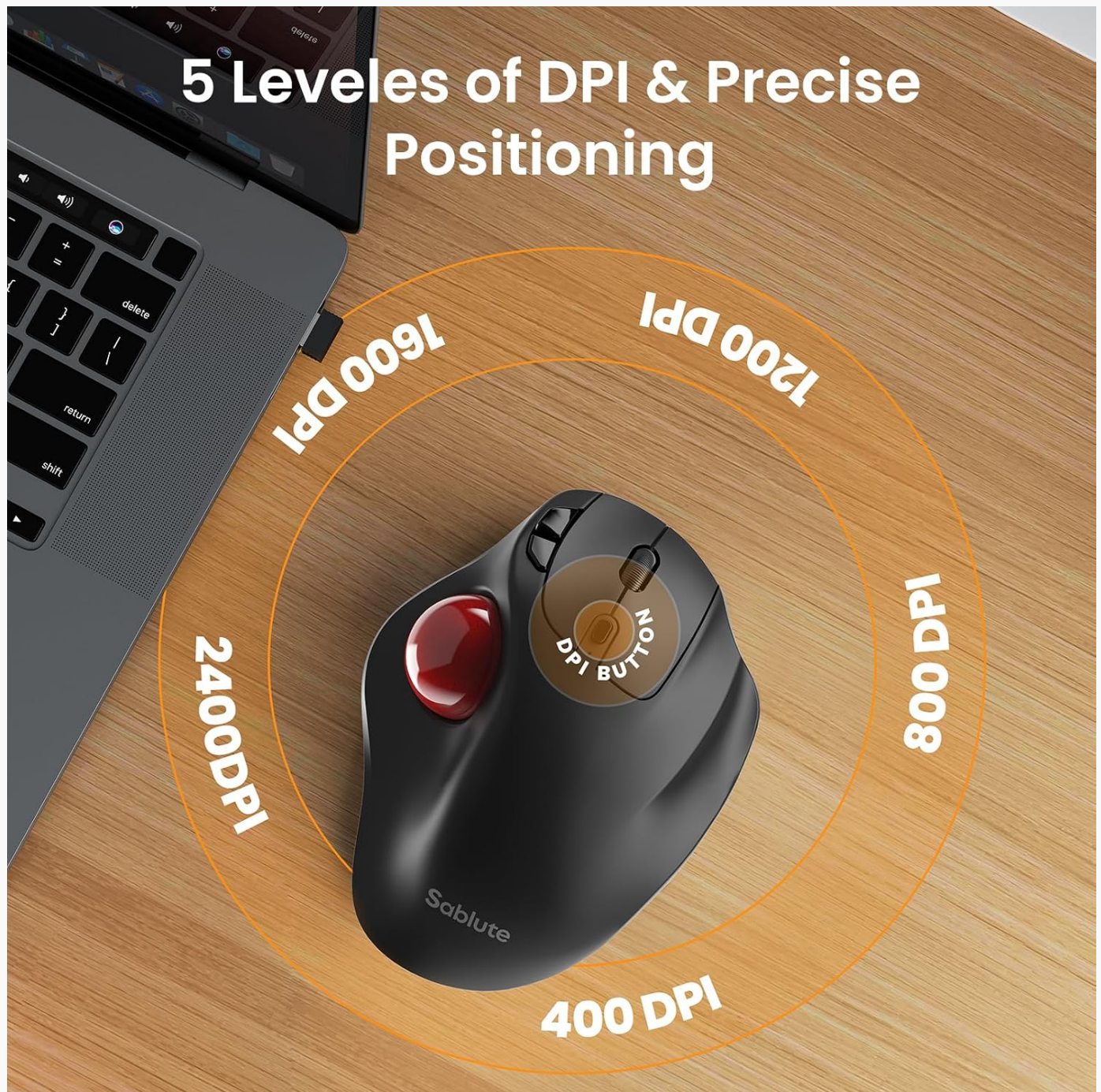
Image: The SABLUTE MAM2 Wireless Trackball Mouse with an overlay indicating the 5 adjustable DPI levels (400, 800, 1200, 1600, 2400) and the location of the DPI button.
