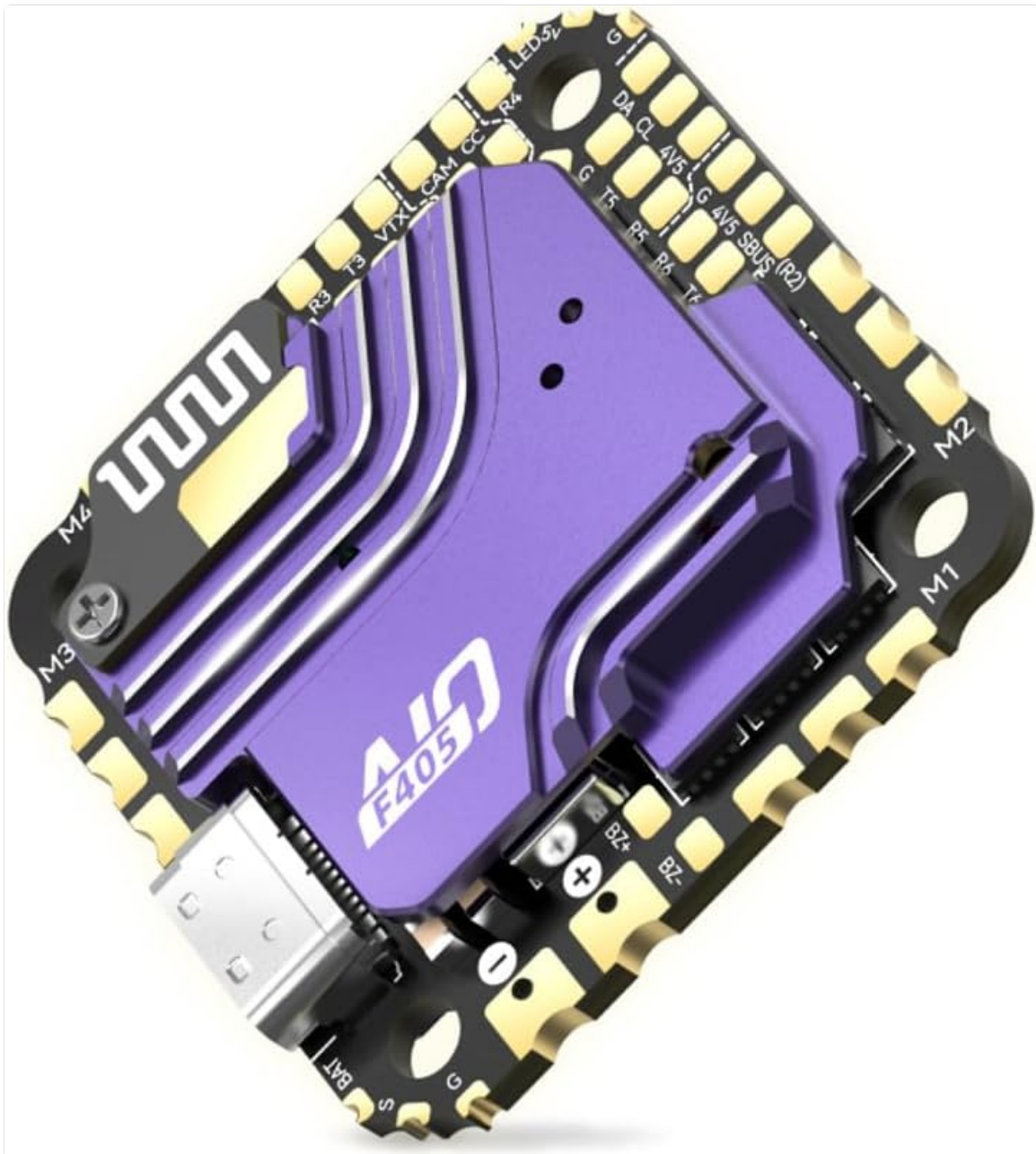
Figure 3: Angled view of the F405 AIO 40A Flight Controller, showcasing the purple heatsink and USB-C port.
