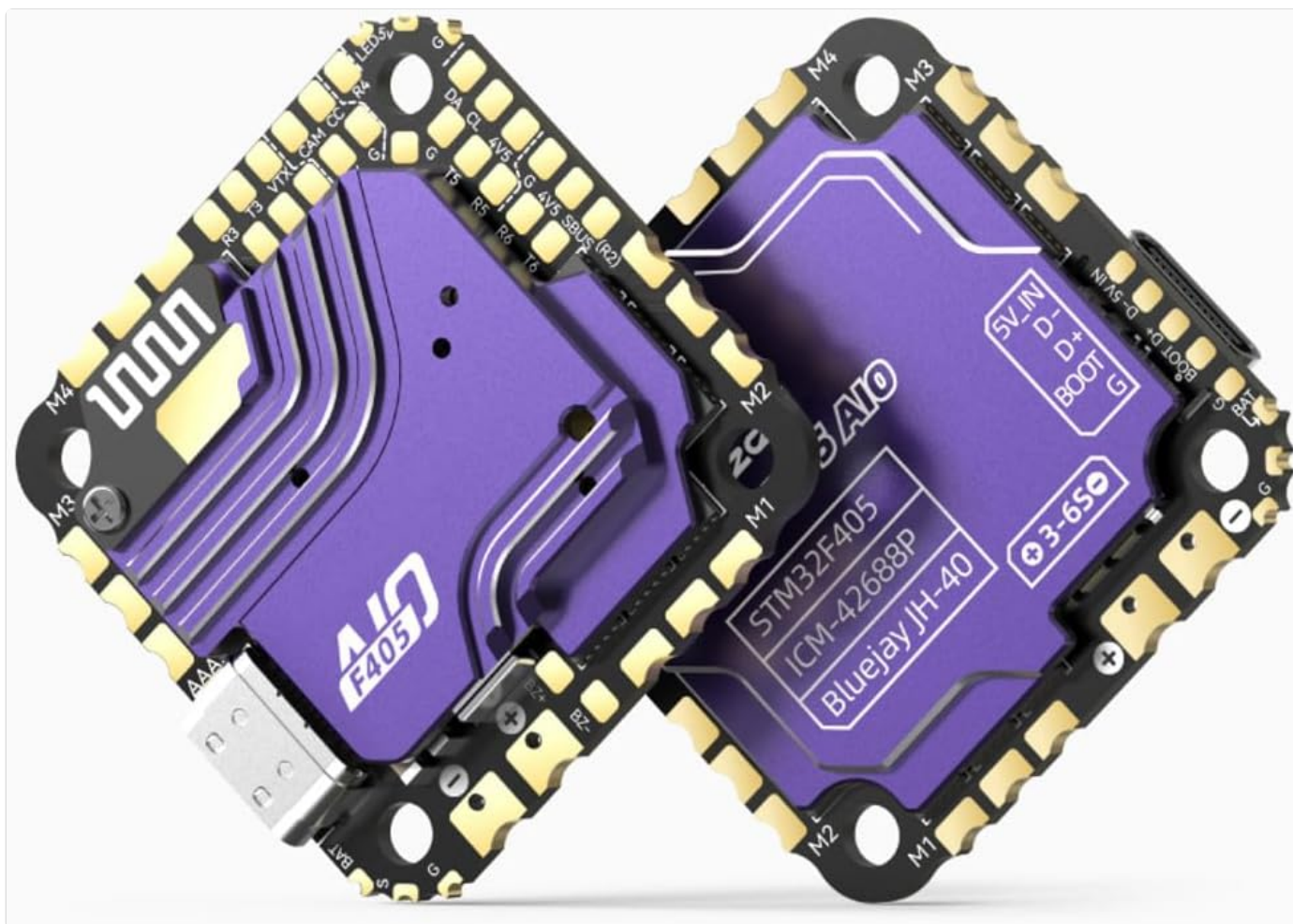
Figure 1: Top and bottom view of the F405 AIO 40A Flight Controller, showing component layout and mounting holes.
