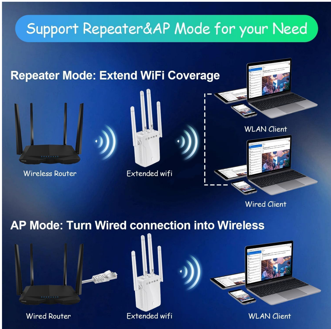
Image: A diagram illustrating the Repeater Mode, where the extender wirelessly extends a router's signal, and AP Mode, where it converts a wired router connection into a wireless signal.
