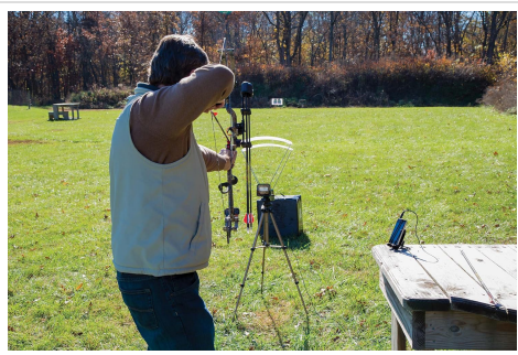
Figure 2: Proper setup of the chronograph for archery, showing the unit on a tripod and connected to a smartphone.
