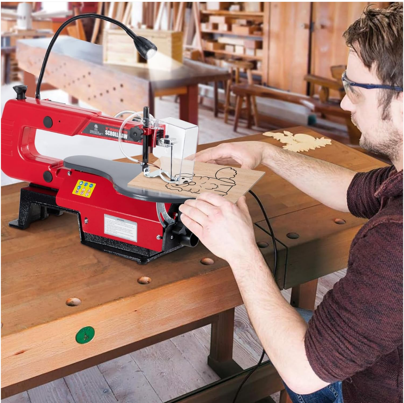
Figure 5.1: A user demonstrating the operation of the scroll saw, carefully guiding a wooden workpiece. This illustrates proper hand placement and focus during cutting.
