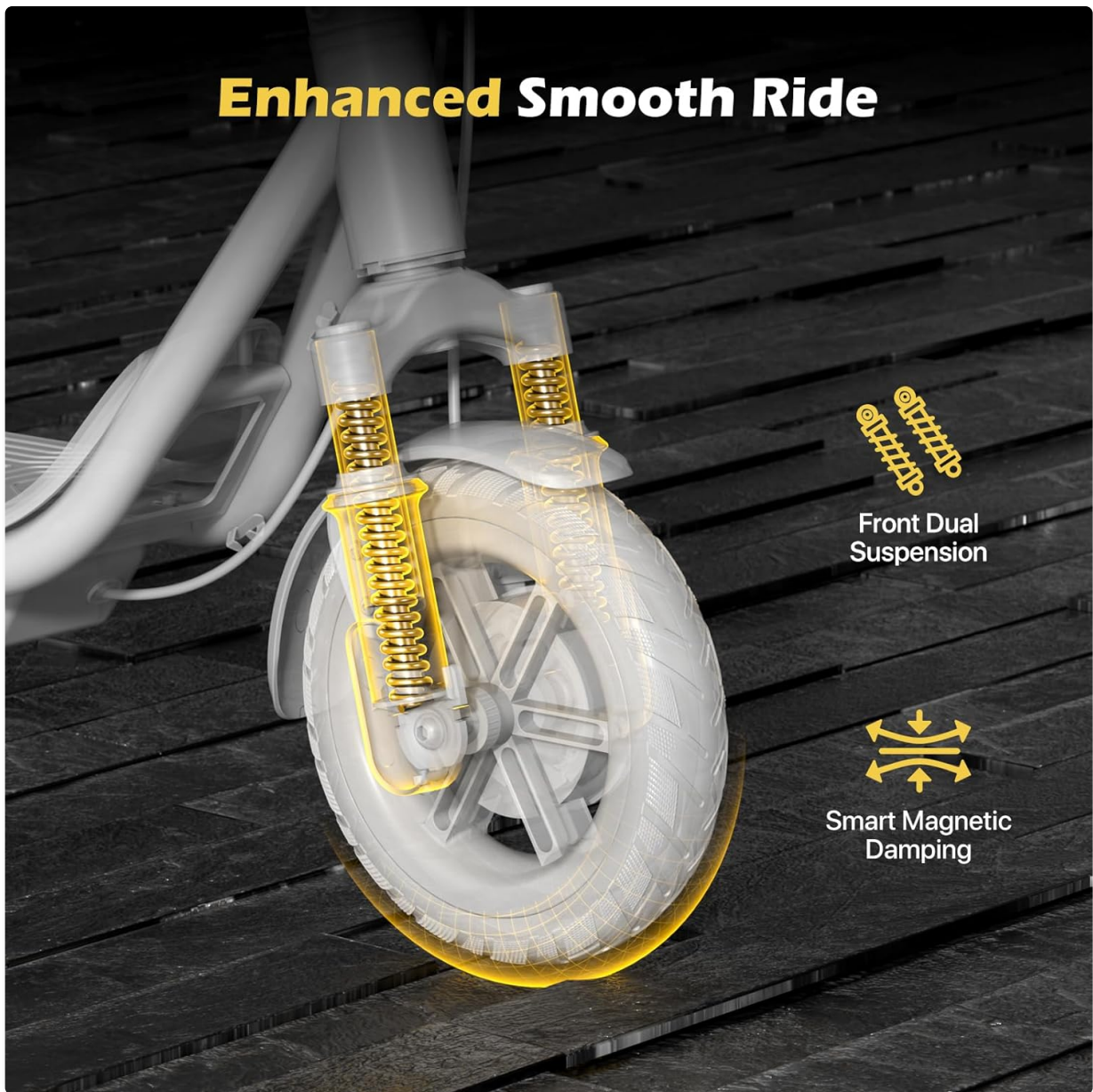
Image 7.1: The front dual suspension system, contributing to an enhanced smooth ride.
