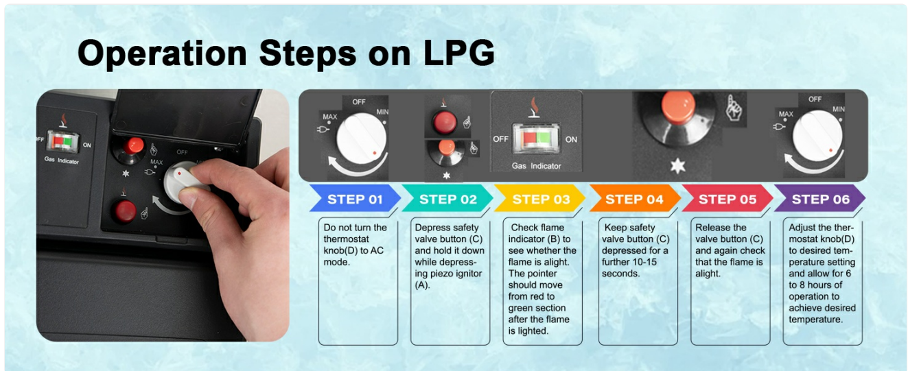
Image: A comprehensive visual guide outlining the six steps required to operate the refrigerator using LPG gas, including ignition and temperature adjustment.
